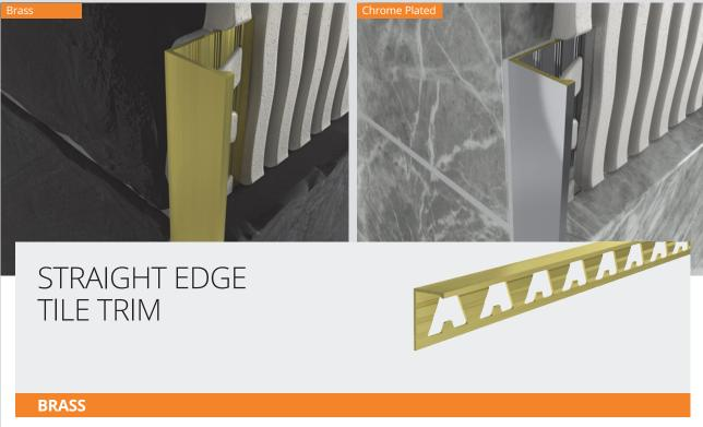
A Brass profile for protecting and finishing tiled corners and edges. Provides a decorative finish and protects adjacent tile edges. Can be used in areas of high mechanical stress. Resistant to most chemicals. Suitable for exterior use. Features a perforated anchoring leg for securing in adhesive or mortar bond below the tiled surface.
